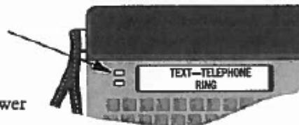
4. When your call is finished, hold down either **Shift** key and press the **TTY On/Off** key to hang up.
