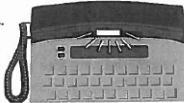
2. Turn on the Uniphone 1140 by pressing the **TTY On/Off** key.
